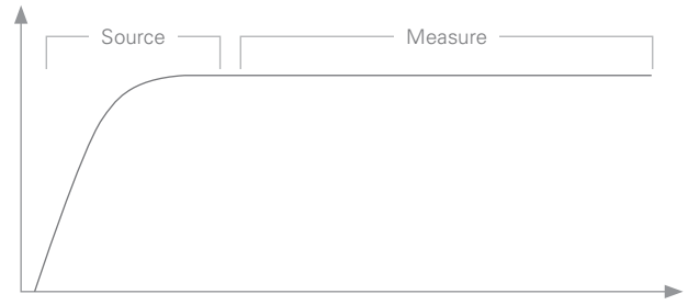
FIG 4 Illustration of the aperture time of an SMU with respect to a sample signal
